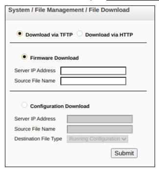
There are 2 methods to upload the firmware file via web interface: using a TFTP server or using an HTTP server.
