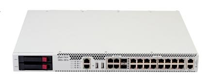
Hybrid platform SMG-3016 is used as a trunk gateway for interfacing of signal and media streams of TDM and VoIP networks. The gateway also might be used as an IP PBX with value added services (VAS) support and a multipurpose solution for infocommunication new generation networks (NGN). The wide function-set, strict compliance with requirements and standards and carrier class reliability allow service providers and carriers to solve most part of their objectives on the basis of SMG-3016.
